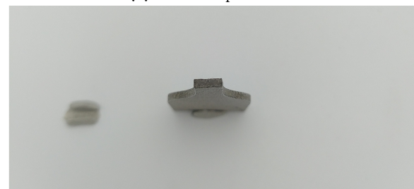
(d) PBF-LB/M specimens fracture surface. Fracture had resemblance to brittle fracture. At the walls seemed to be a gap.
