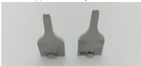
(c) Rolled sheet metal specimens fracture surface. Ductility was clearly visible.
