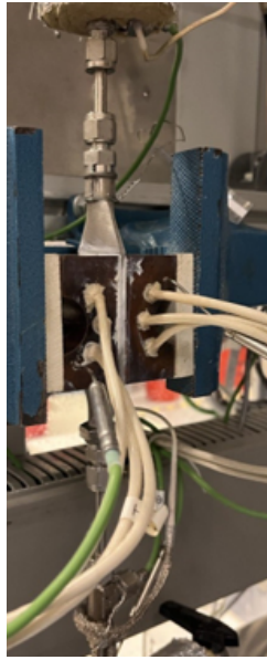
(a) Photo of module. Note distance between thermocouples (in T-pieces) and inlet/outlet.
