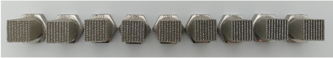
(a) Frit modules with HD increasing from left to right.
