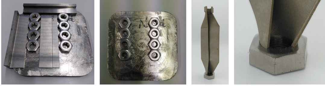
Figure 4.6.: Hybrid manufacturing of modules on nuts with exemplary empty module (three-quarter cut).
