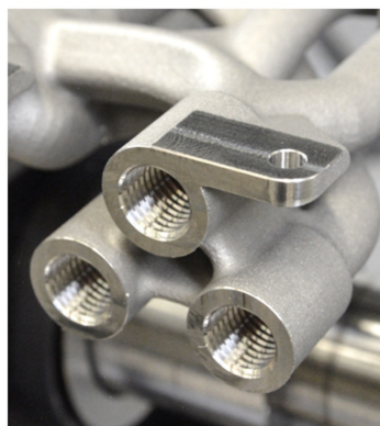
Figure 3.11.: Photo of PBF-LB/M threaded holes [217].
