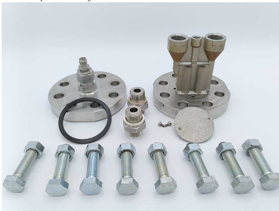
(c) Hybrid reactor with counterflange and accessories.
