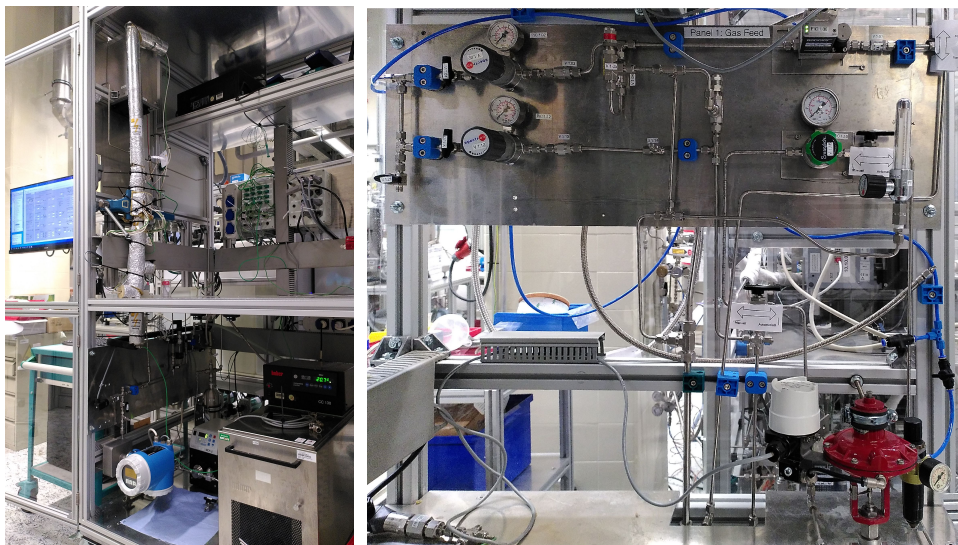
(a) Left side containing water circuit and (b) Right side containing N 2 supply, system pressure control, and mass-flow controller for pressure difference testing in section 4.2.
