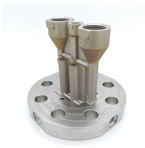
(b) Hybrid reactor after post-processing. Note different surface of conventionally and additively manufactured sections.
