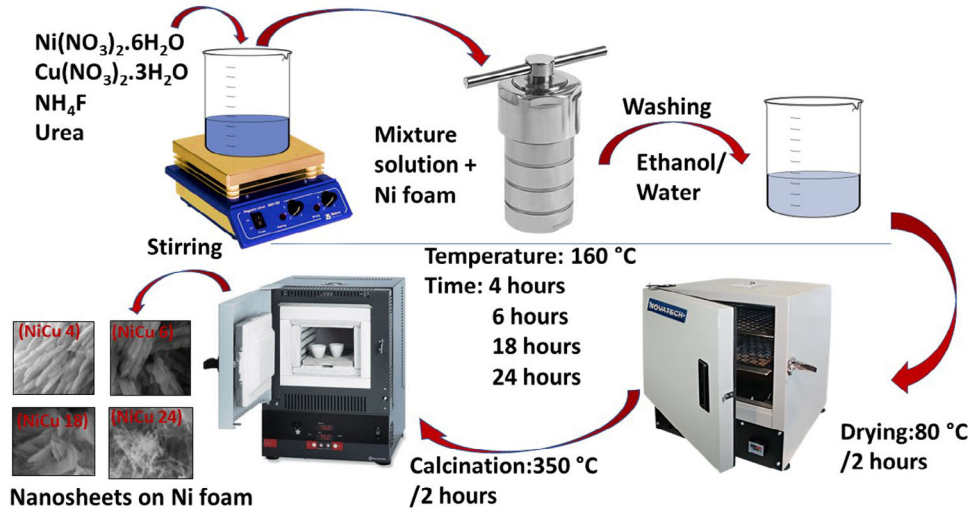
Figure 1. Schematic diagram for fabrication of Ni-Cu bimetallic oxides with various growth time.
