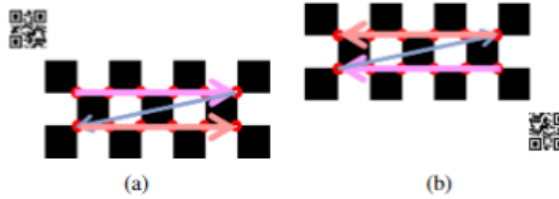
Figure 5.3: To overcome the directional challenge associated with the feature points on the calibration patterns, the corner detection process commences from the corner closest to the QR code and advances in a sequential manner along rows and subsequently columns.
