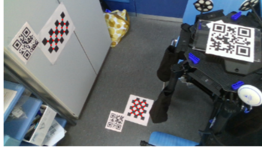
Figure 5.7: Reprojection of the identified corners of the calibration patterns from the RGB-D camera rig onto the image plane of the external camera.
