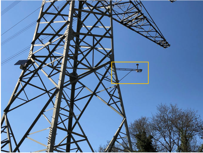
Figure 2.1: Field tests were conducted along two high-voltage lines as part of the PrognNetz project to gather crucial ambient weather data required for artificial intelligence-based power load forecasting. The weather stations, indicated by the yellow rectangular boxes, were manually installed on one of the corner legs of the mast by trained technical personnel who climbed the towers following comprehensive safety training.
