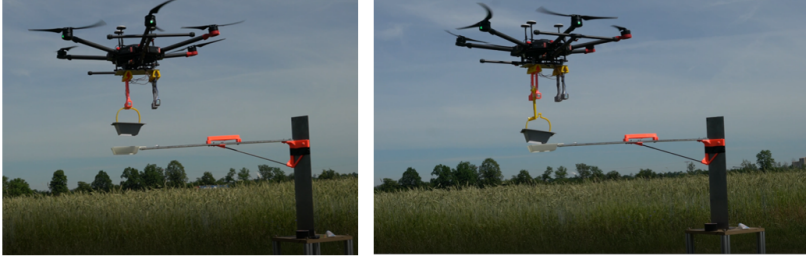
Figure 3.13: The release of the weather station is executed employing the solenoid-based gripper, while the subsequent dismantling process is facilitated through the utilization of the hook-shaped gripper.
