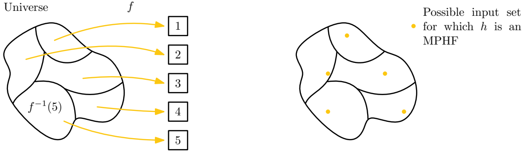
■ Figure 2.6 Preimages of a minimal perfect hash function and a possible input set that the function is minimal perfect on.
