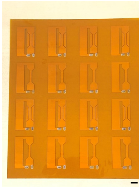
Figure 6.4: an array of fold-up stripline coils ordered from a vendor (MultiPCB, China) before folding. The coil consists of three sandwiched layers: 25 \mu\text{m} PI cover layer, 18 \mu\text{m} copper traces, and 25 \mu\text{m} PI substrate. (scale bar: 5mm)
