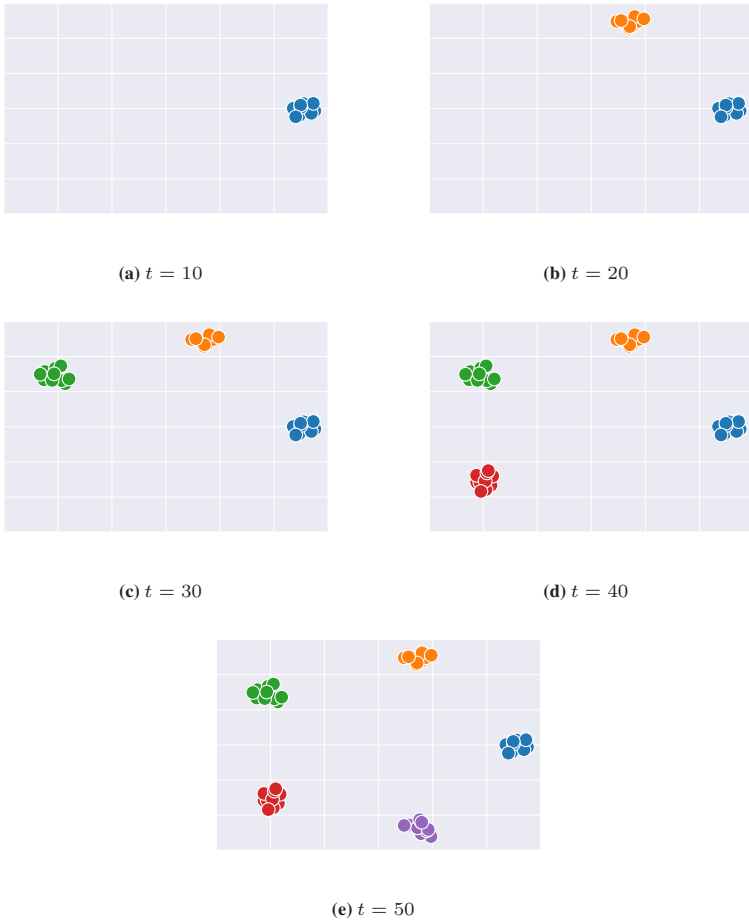
Figure 6.1: Example data from an orbital dataset at different time steps t , for C = 5 and P = 10 . Once P points have been drawn from one component, the next component is sampled. Components are colored to facilitate their identification.
