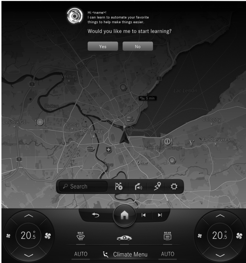
Figure 5.2: Snapshot of the system’s initial UI design. The self-learning system requests user permission to start learning and automating comfort features.
