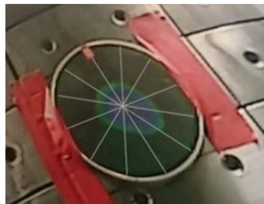
Fig. 3. Hot test with ~1 ms gyrotron pulse at inner torus wall onto a liquid crystal foil target.
