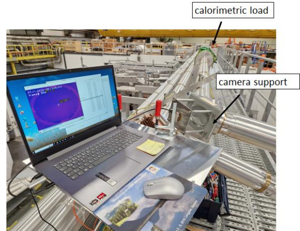
Fig. 12. Miter bend IR detector mounted at the first miter bend of an AUG CWTL.
