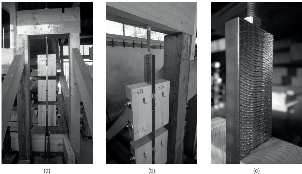
Figure 7.19: Setup of tests with bolts (a+b) and milled steel plate (c).
