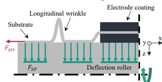
Fig. 1 Schematic of a longitudinal wrinkle in an electrode at the deflection roller according to [8] with an additional stretching force  $F_{str}$
