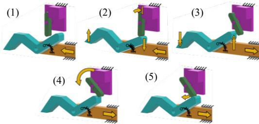
Fig. 6 Motion sequence of the finger gripper, shown for one finger only for clarity
