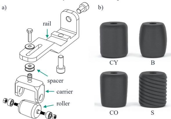
Fig. 3 a) Roller holder, b) Roller geometries: cylindrical (CY), barrel-shaped (B), conical (CO), cylindrical with spiral profile (S)
