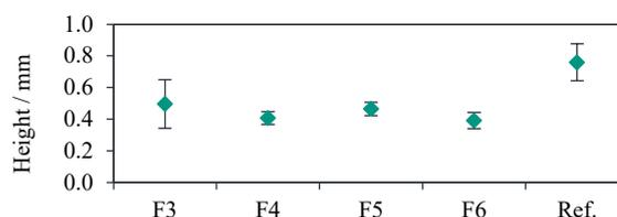
Fig. 11 Change in the height of the longitudinal wrinkles over the different test parameters and reference without intervention of the finger grippers (Ref., Experiment no. #6 from [8])
