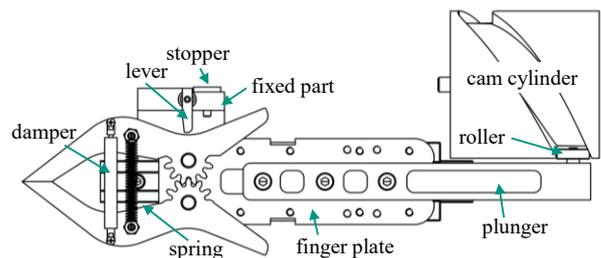
Fig. 5 Sketch of the finger gripper system
