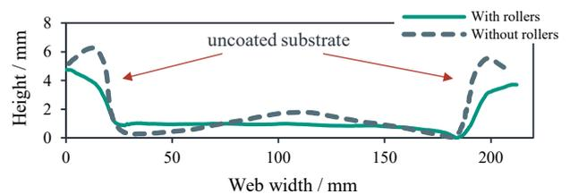
Fig. 8 Averaged cross-section in x-direction through the laser data of the calendered NMC811 electrode with and without additional rollers
