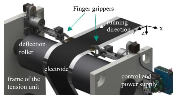
Fig. 4 CAD model of the entire finger gripper concept
