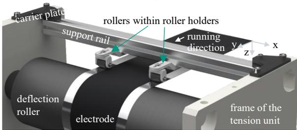
Fig. 2 CAD model of the entire roller concept
