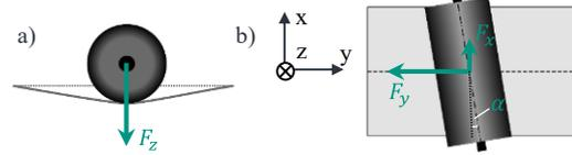
Fig. 7 Installation situation of the rollers in the experiment
