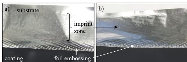
Fig. 9 Longitudinal-wrinkle-free calendered electrodes: a) conical rollers, b) spirally profiled roller
