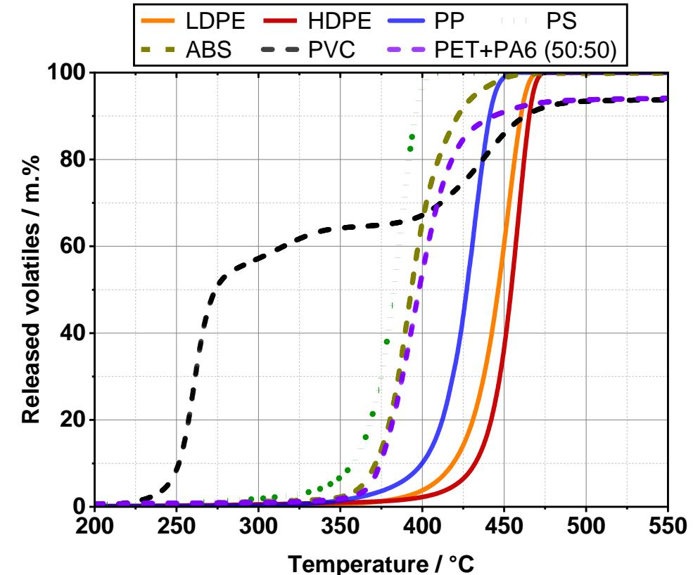
→ Accelerated PET and PA6 degradation may improve temperature staging effect
