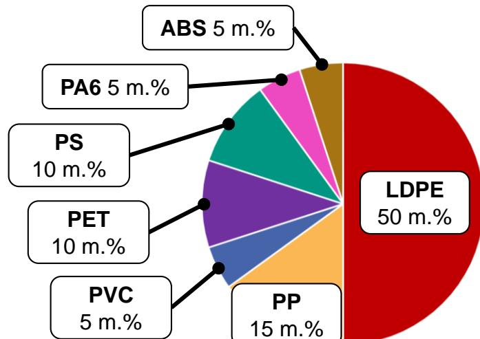
Thermoplastic mixture with high amount of N-, O- and Cl-containing polymers
