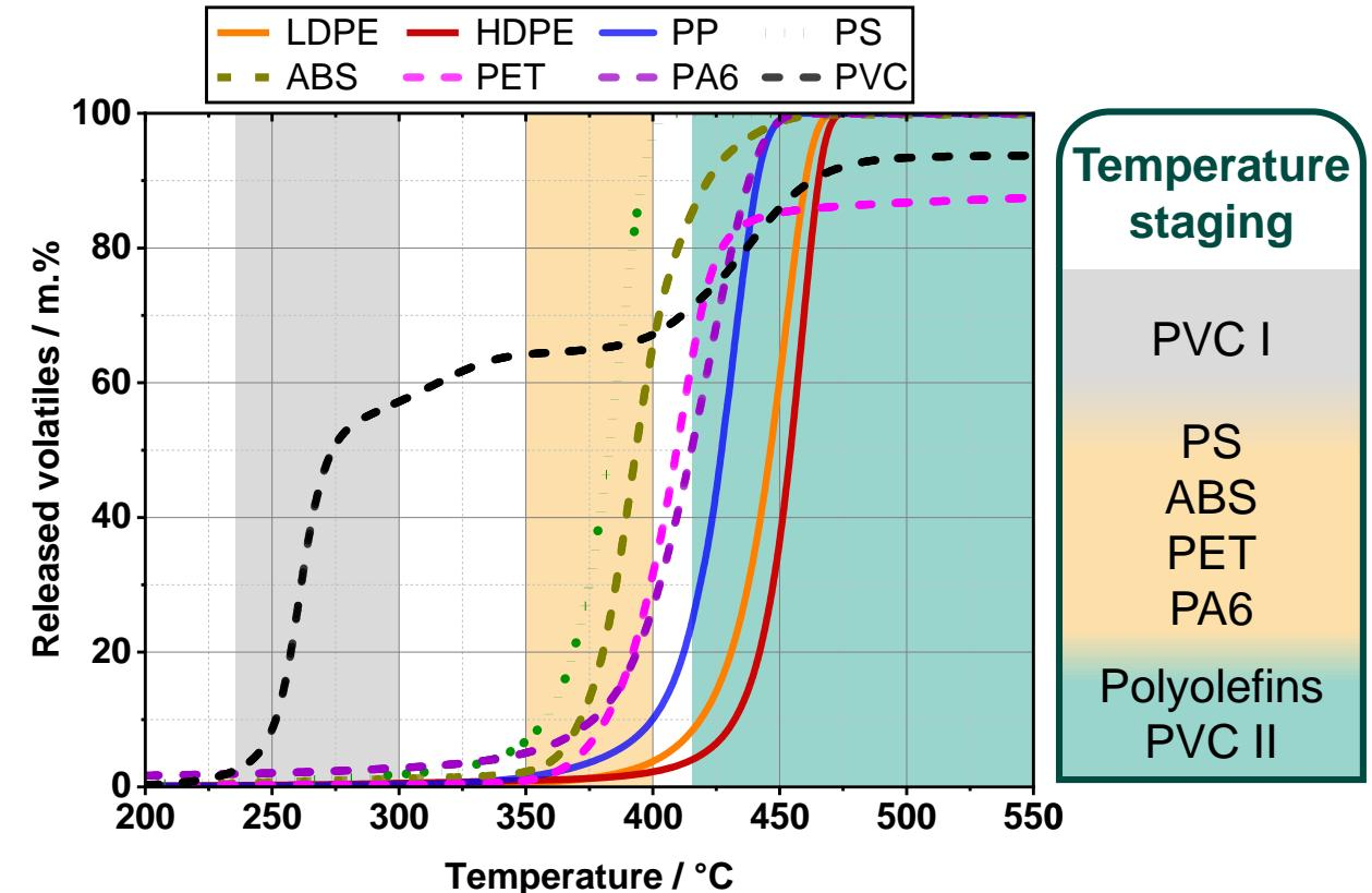
→ Reaction rate at specific temperatures differs by polymer type
