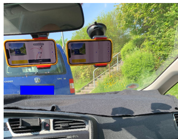
Figure 4 Exemplary sensor setup used to record the dataset.
