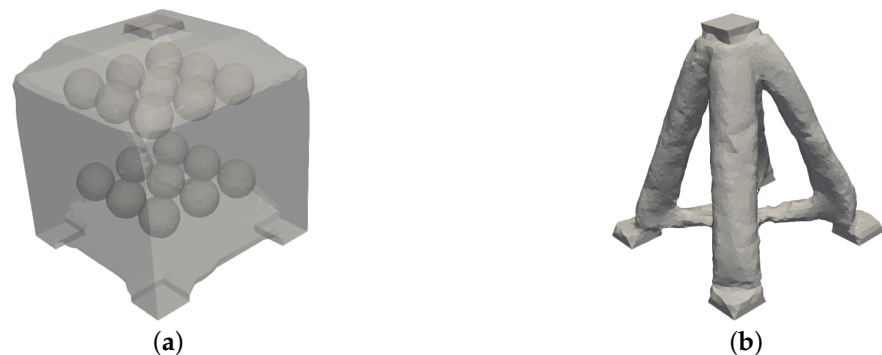
Figure 13. (a) Initial hole structure of the box in the single-material case. (b) Optimization result for the box at iteration 107.
