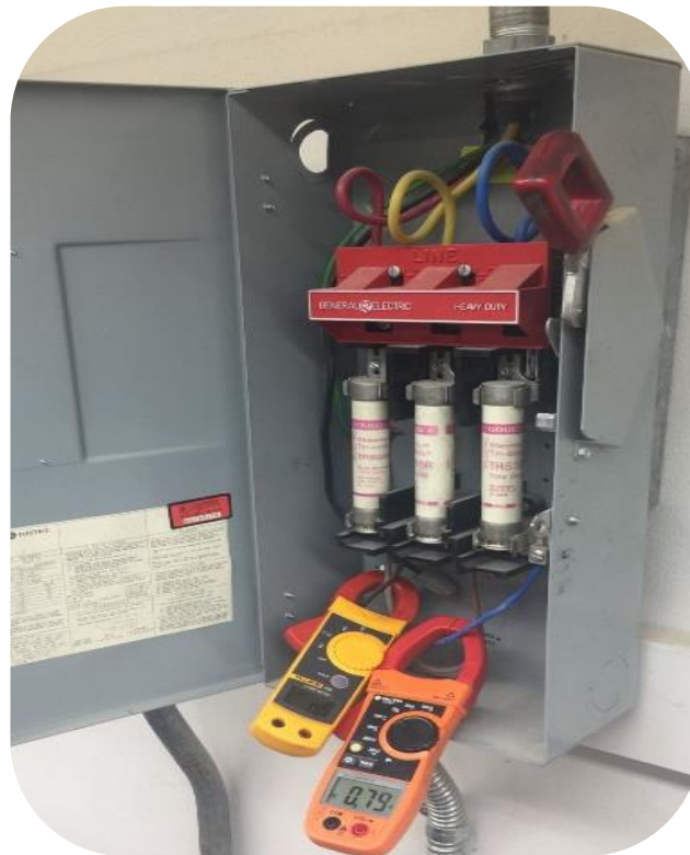
Figure 5. Test rig for power consumption measurement.
