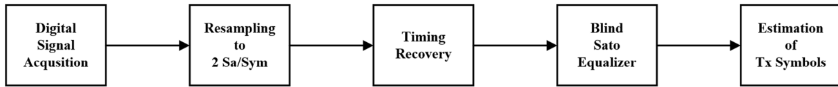
Figure 4. Digital signal processing chain to recover the transmitted waveform. After signal reception using a digital storage oscilloscope, resampling to two samples per symbol is carried out. The following feed-forward timing recovery and a subsequent blind Sato equalizer allow to reconstruct the transmit (Tx) symbols. Evaluation is then performed in terms of constellation signal to noise ratio and bit error ratio.
