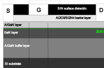
Typical structure of a GaN HEMT
