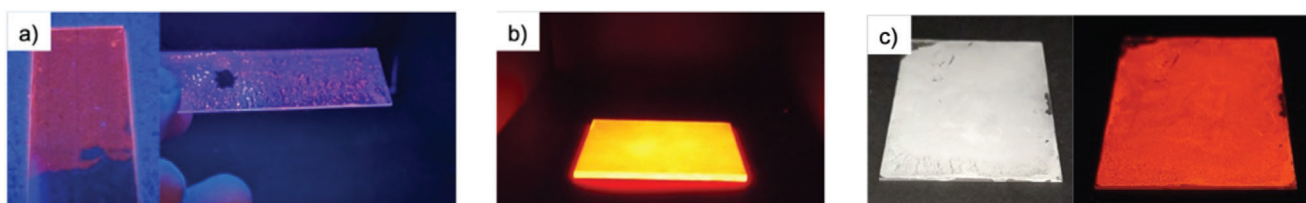
Figure 7. Photographs of the development of the paint samples using compound 13 on borosilicate glass with a) polypropylene-based paint, b) acrylic-based paint, and c) in commercial whitewash (left – ambient light; right – under UV). All samples are under 302 nm UV light.
