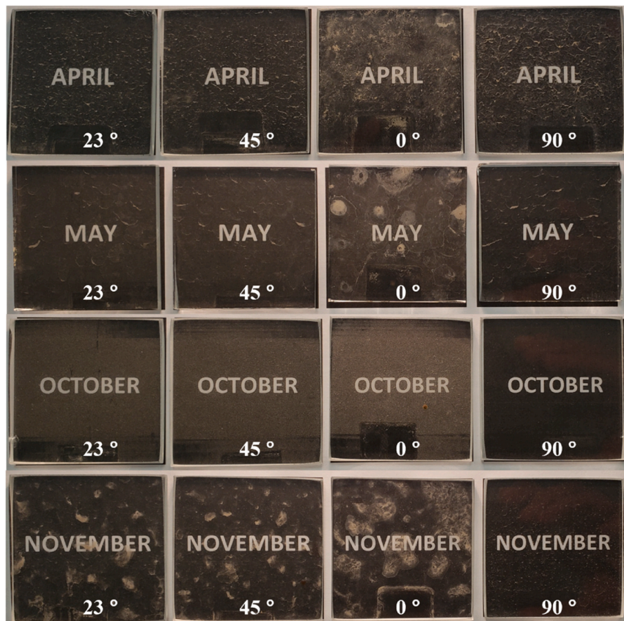
Fig. 8. Photographs showing sixteen samples of soiled glass coupons collected for the months of April, May, October and November, and at four orientations each. These months were selected to show the overall variation in dust depositions over the course of the present (annual) investigation.
