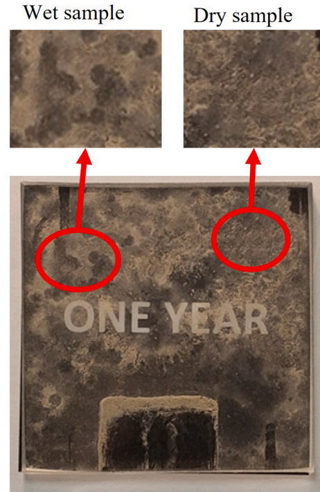
Fig. 13. Illustration of soiling distributions for the one-year horizontal sample demonstrating a similar pattern to the patterns captured separately during wet and dry seasons.
