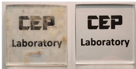
Fig. 5. Photographs showing the one-year horizontal sample at the end of the study period (left) alongside a clean glass coupon (right).
