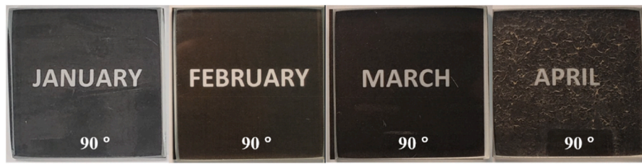
Fig. 11. Vertical soiled coupons for January, February, March and April. The measured average transmittance was 77 %, 82 %, 82 %, and 61 %, respectively.
