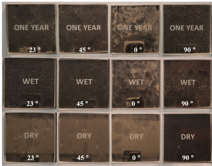
Fig. 7. Photographs showing twelve glass samples of collected soiled glass coupons for different seasons (wet and dry seasons) and for the whole year at four different tilt angles: 0°, 23°, 45° and 90° (the backgrounds of the photographs are pure black).
