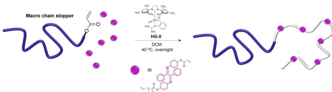
Figure 3.1. Synthesis of photoswitchable block copolymer via head-to-tail ADMET polymerization featuring main-chain \alpha -bisimine photoswitch.
