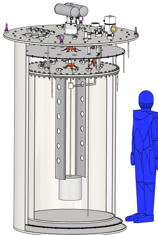
(b) Cryostat mechanical design
