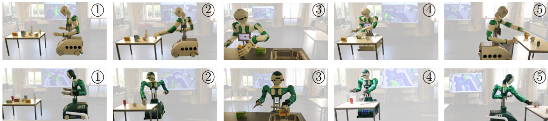
Figure 5.3.: Table-clearing of known and unknown objects with ARMAR-DE and ARMAR-6 . ① Initial setup, ② grasping of known objects, ③ placing of known objects, ④ grasping of unknown objects, and ⑤ placing of unknown objects.
