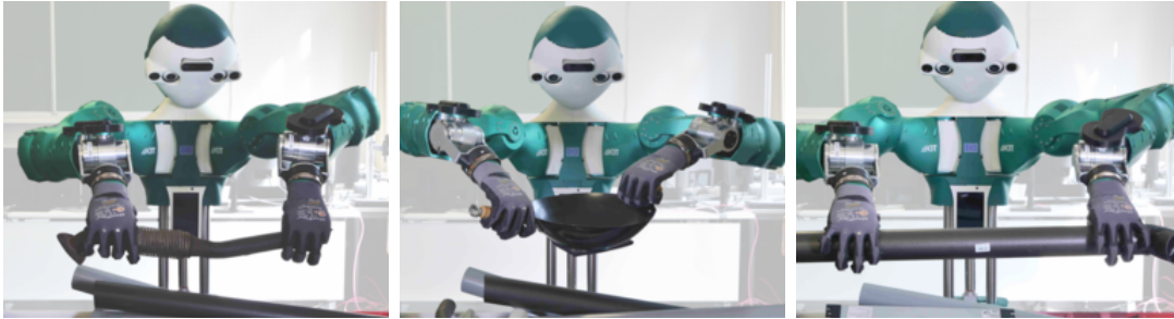
Figure 5.4.: The humanoid robot ARMAR-6 grasping and carrying multiple objects (exhaust, pan, and pipe) bimanually.
