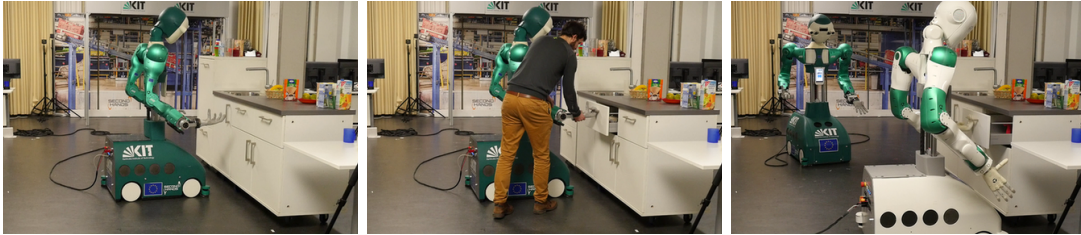
Figure 5.5.: Transfer of drawer- opening skill, which was learned through kinesthetic teaching, from ARMAR-6 to ARMAR-DE .
