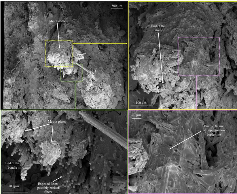
**Figure 5.23:** SEM pictures of the fracture surface of the  $0^\circ$  CF<sub>LFT</sub> flow specimen from Figure 5.21 at the point of local strain increase marked in Figure 5.21 in different magnifications.
