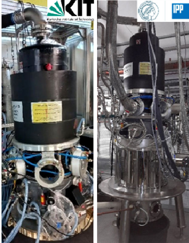
Figure 1. TH1507U prototype under test at KIT (Left) and the unit installed at IPP (Right).
