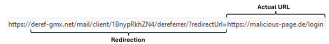
Figure 8. Legitimate redirects by an email provider are misused here to disguise the destination malicious-page.de . Users who follow common security awareness training (Reinheimer et al., 2020) may only check the derefer-gmx.net part of the URL, unaware that it actually redirects to malicious-page.de .
