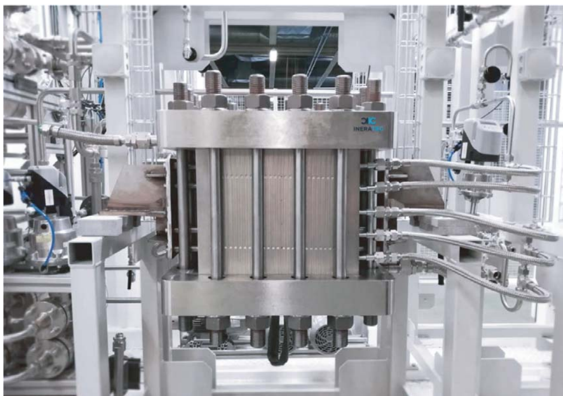
Fig. 8 Approved 2 bpd reactor module from INERATEC GmbH inside the skid of a 1 MW(el) PtL plant [71] (bpd: barrel per day)
