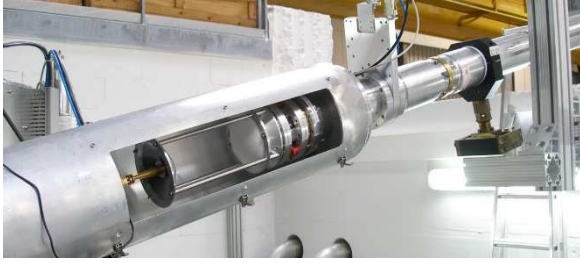
Fig. 3. Lens horn mounted at the input of a ASDEX Upgrade waveguide transmission line.
