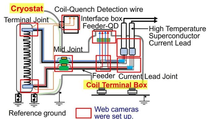
Figure 5. Schematic view of global Paschen test.
