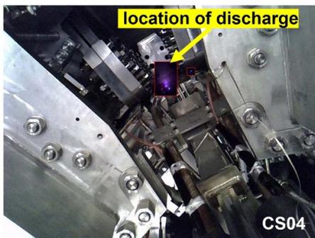
Figure 7. Overlapping of discharge image onto the actual configuration.
