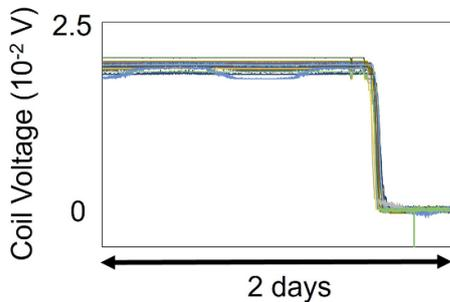
**Figure 13.** Transition to superconducting state (TF coils).
