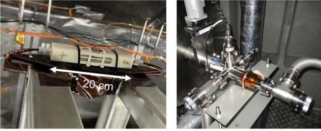
**Figure 11.** Cold cathode gauge (left: EU, right: JA).
