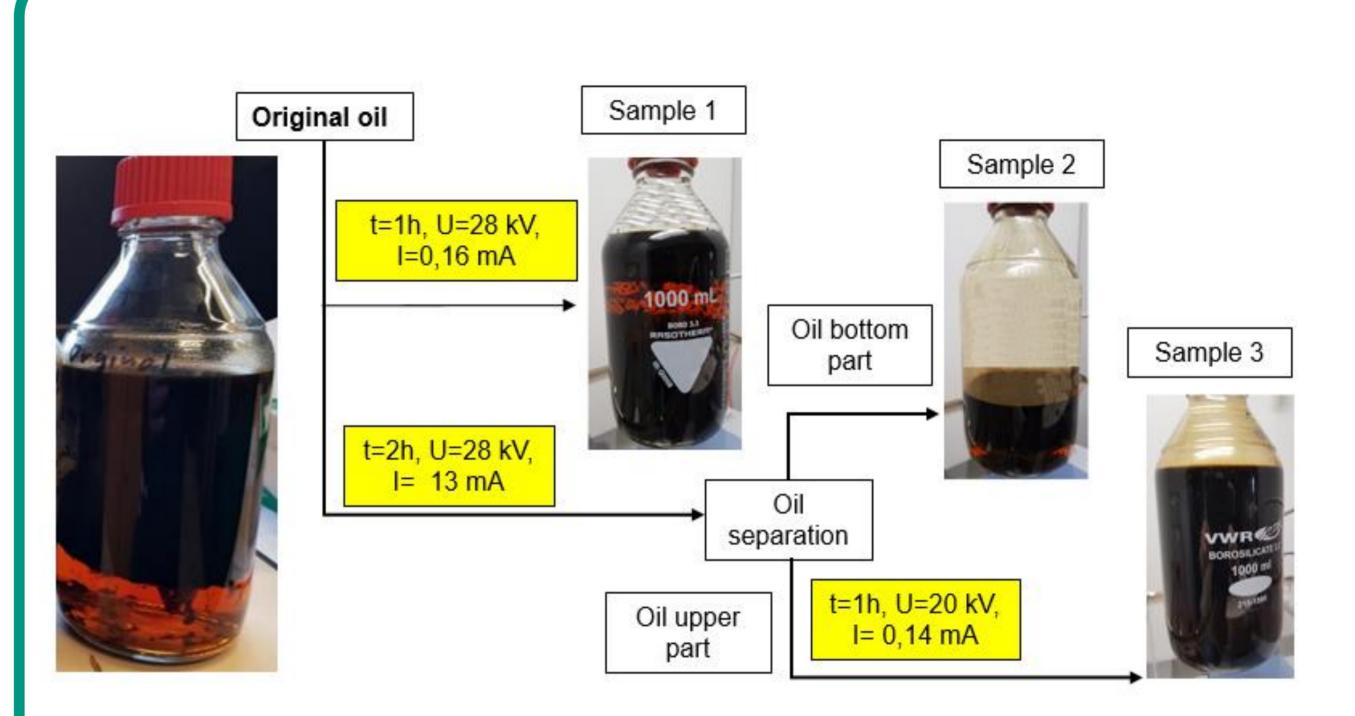
EHD treatment in a DC corona discharge of pyrolysis oil, collected from a condensation system of the pyrolysis reactor for plastic wastes.
