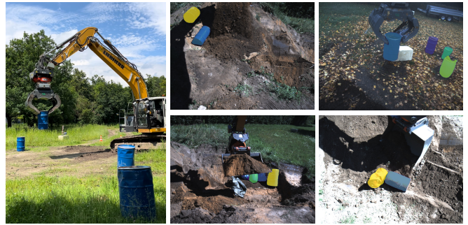
Fig. 5: Excavator ALICE grasping barrels (left) using panoptic segmentation masks (right) obtained from a Mask2Former [60] model trained on the GOOSE-Ex dataset.
