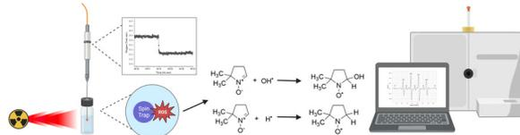
Figure 1: Schematic of the measurement process: irradiation, real-time O<sub>2</sub> measurement and post-irradiation spin-trapping spectrum measurement.
