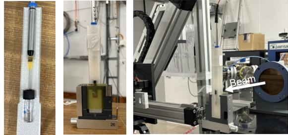
Figure 2: Experimental setup: Sample with oxygen sensor, dosimetry configuration using film dosimeter and complete setup at the accelerator.
