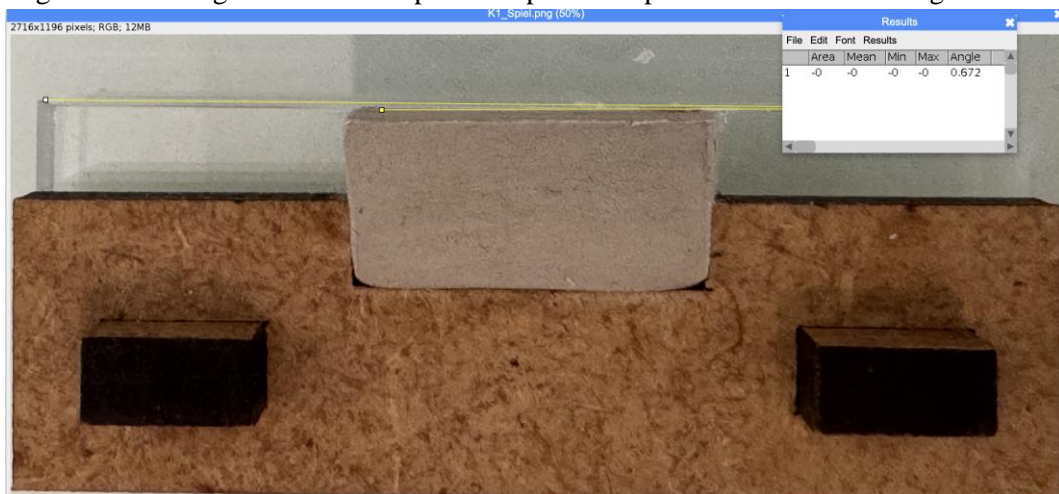
Figure 13. Testing result of Concept 1 with clearance deviation 2mm: Coin angle = 0.67^\circ
