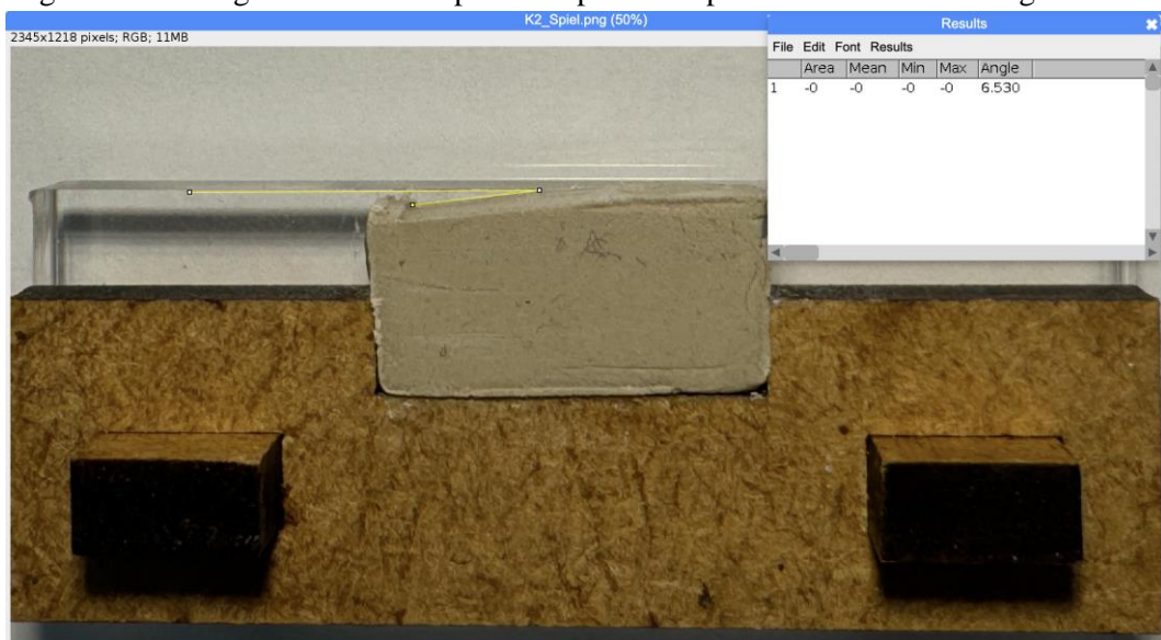
Figure 16. Testing result of Concept 2 with clearance deviation 2mm: Coin angle = 6.53^\circ
