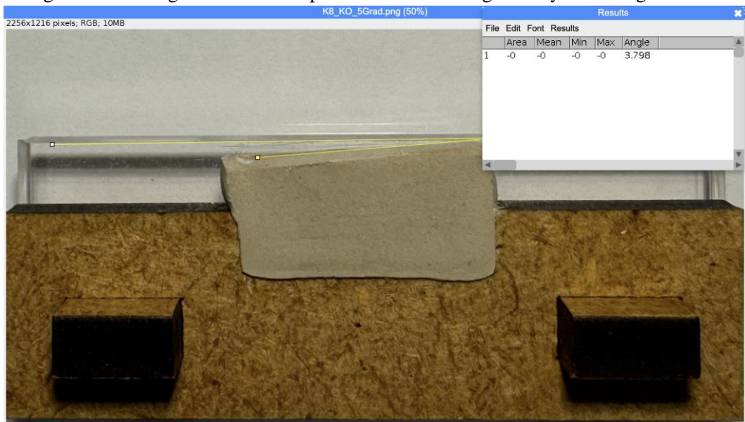
Figure 33. Testing result of Concept 8 with piston shape deviation 5^\circ : Coin angle = 3.80^\circ
