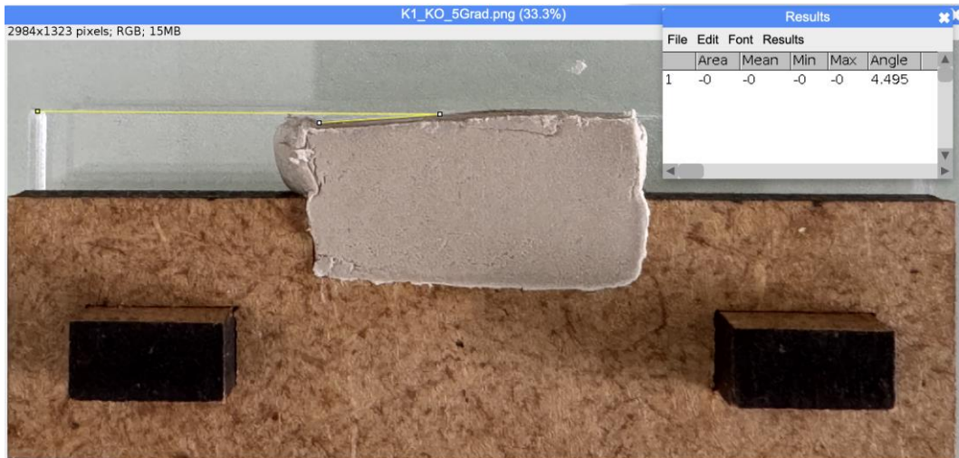
Figure 12. Testing result of Concept 1 with piston shape deviation 5^\circ : Coin angle = 4.50^\circ
