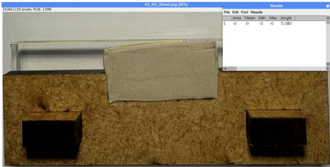
Figure 15. Testing result of Concept 2 with piston shape deviation 5^\circ : Coin angle = 5.08^\circ
