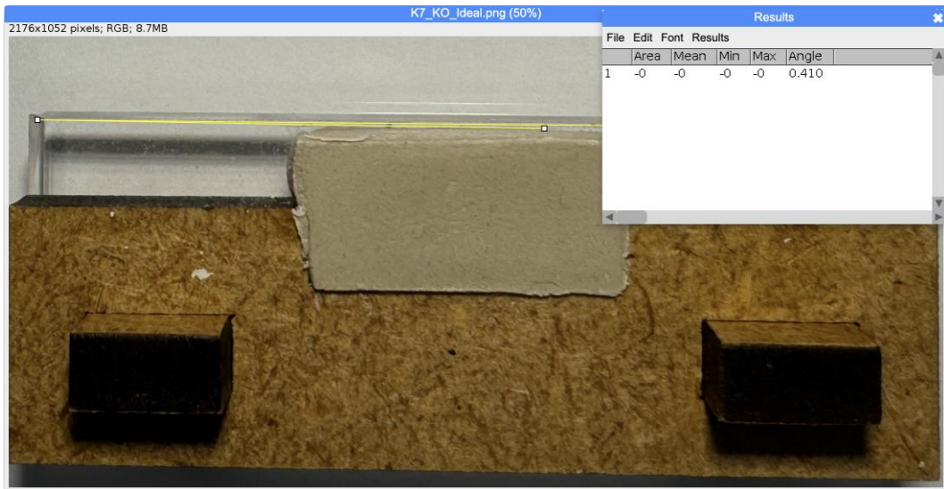
Figure 29. Testing result of Concept 7 with ideal CAD geometry: Coin angle = 0.41^\circ
