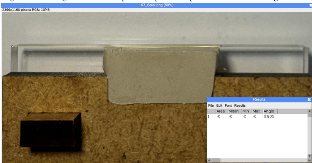
Figure 31. Testing result of Concept 7 with clearance deviation 2mm: Coin angle = 0.91^\circ
