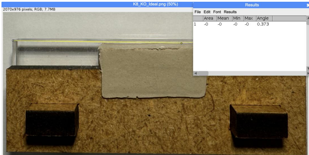
Figure 32. Testing result of Concept 8 with ideal CAD geometry: Coin angle = 0.37^\circ
