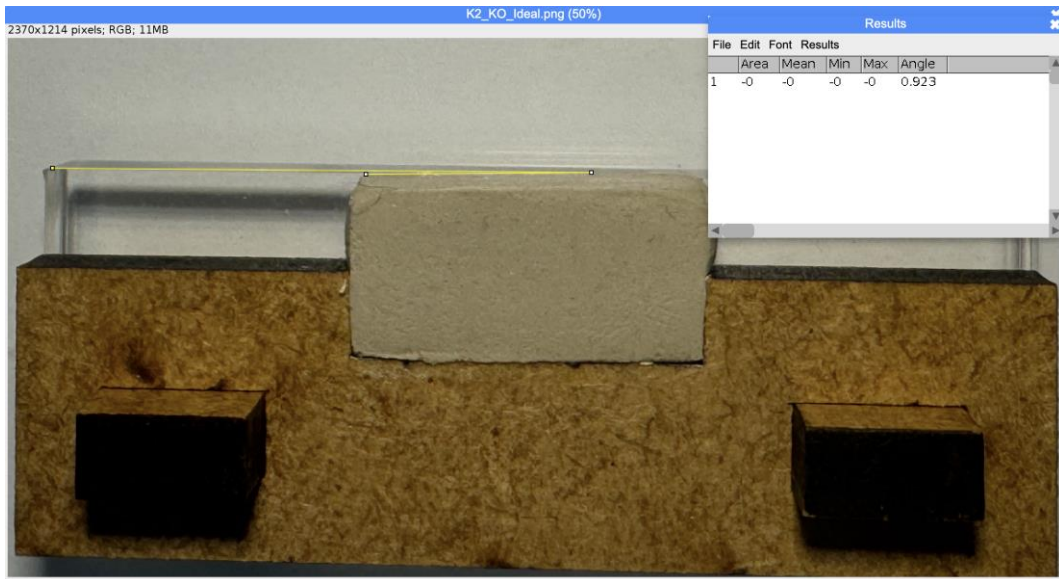
Figure 14. Testing result of Concept 2 with ideal CAD geometry: Coin angle = 0.92^\circ
