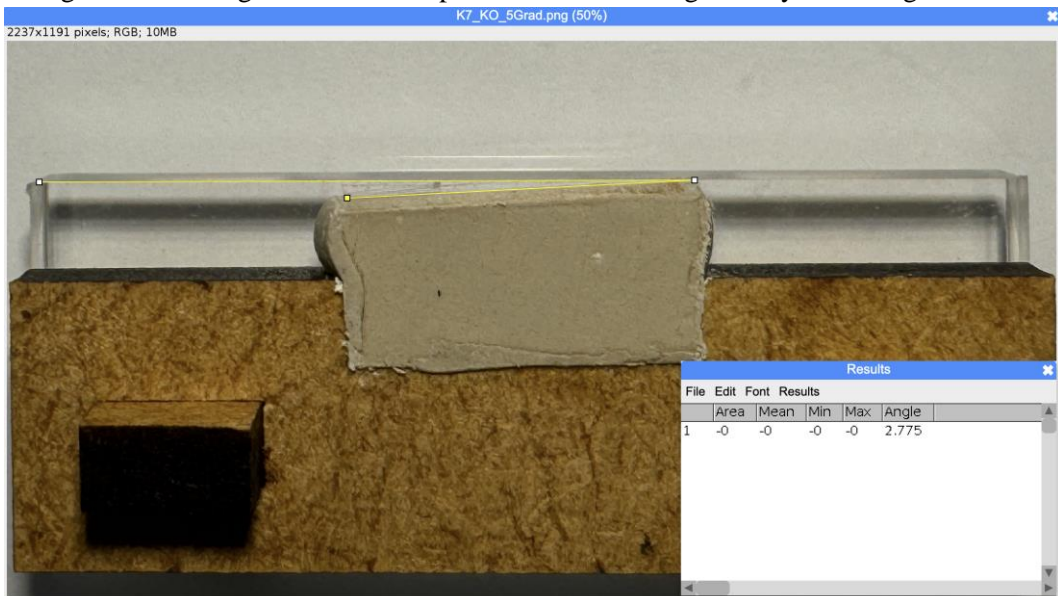
Figure 30. Testing result of Concept 7 with piston shape deviation 5^\circ : Coin angle = 2.78^\circ
