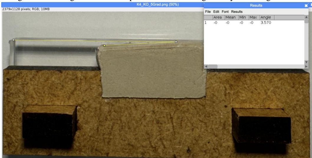
Figure 21. Testing result of Concept 4 with piston shape deviation 5^\circ : Coin angle = 3.57^\circ
