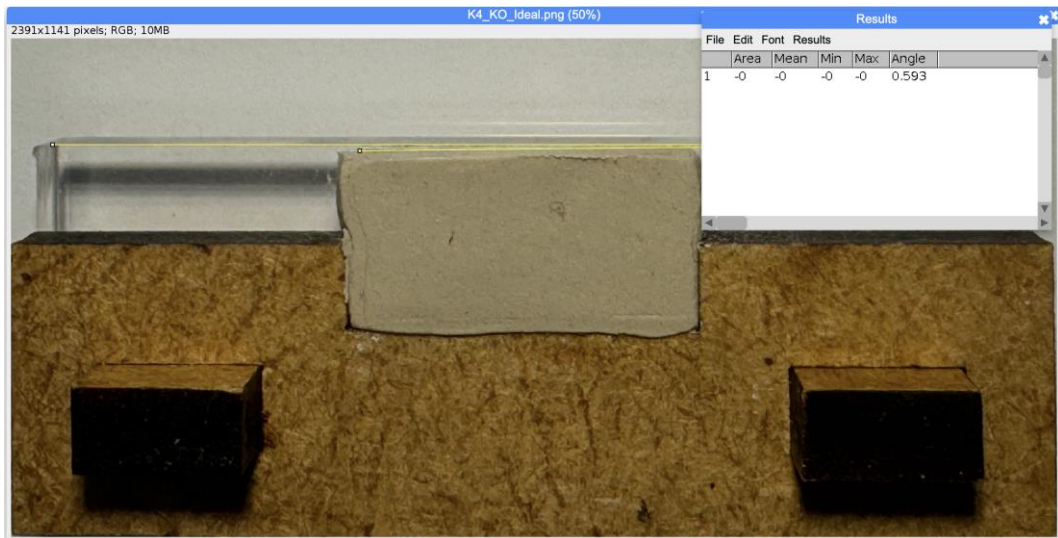
Figure 20. Testing result of Concept 4 with ideal CAD geometry: Coin angle = 0.59^\circ
