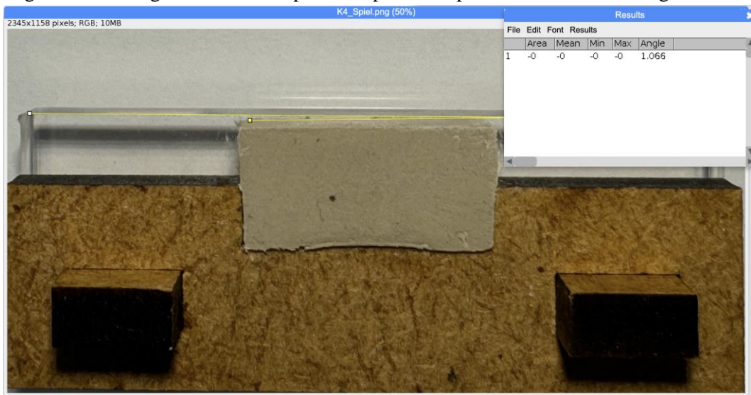
Figure 22. Testing result of Concept 4 with clearance deviation 2mm: Coin angle = 1.07^\circ
