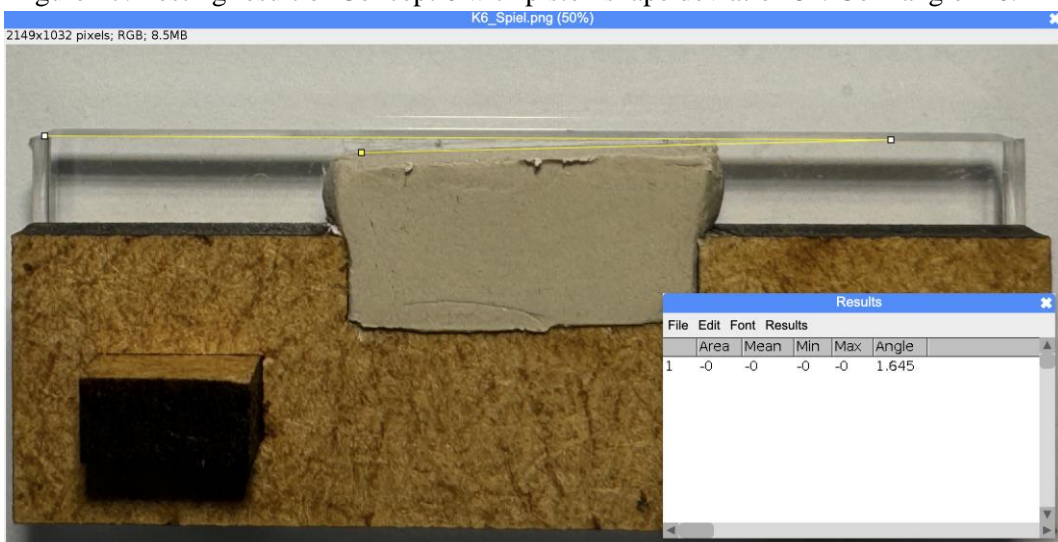
Figure 28. Testing result of Concept 6 with clearance deviation 2mm: Coin angle = 1.65^\circ
