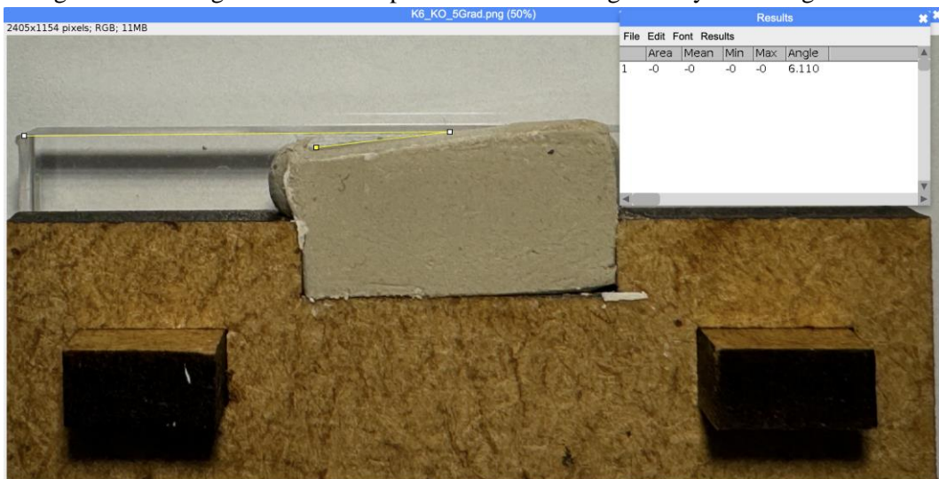
Figure 27. Testing result of Concept 6 with piston shape deviation 5^\circ : Coin angle = 6.11^\circ
