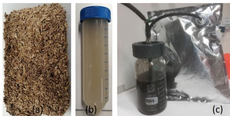
Fig. 29: (a) Dried beer marc (b) wood juice (c) fermentation sample in a 1 l glass reactor with gas bag for biogas collection
