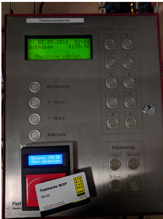
Figure 4.1.: Test Setup: A Vending Reader (lower left) embedded into a washing machine controller
