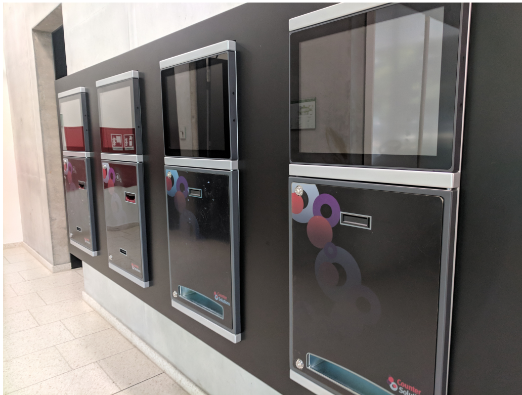
Figure 7.1.: Revalue devices secured by a solid enclosure
