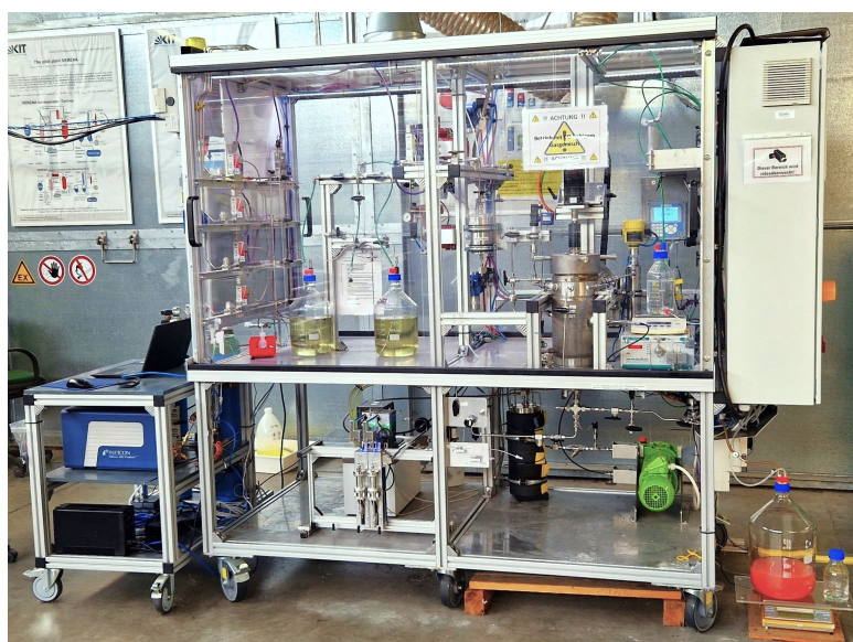
Figure A.11: Final experimental setup for continuous fermentation of synthesis gas with an external circuit for the retention of biomass and the possibility of operation at increased process pressures. Released in June 2022. Longest time of operation achieved: 3097 hours ( ZpH-I ).
