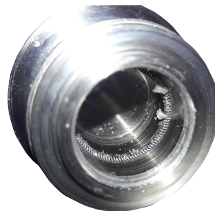
(c) Particle attrition on the spring groove
