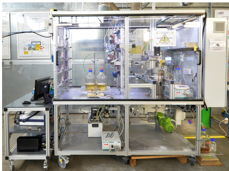
Figure A.10: Further developed experimental setup for continuous fermentation of synthesis gas with an external circuit for the retention of biomass and the possibility of operation at increased process pressures. Released in November 2021. Longest time of operation achieved: 1970 hours ( ZP-II ). Photography: T. Zevaco, 2021.
