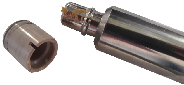
(a) Friction bearing running dry
