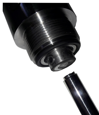
Figure A.13: Breakage of the agitator shaft at the interface to the coupling system after 392 hours of operation.
