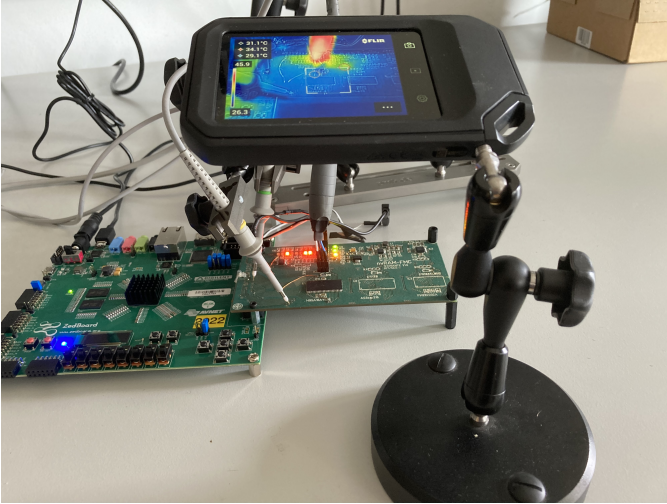
Fig. 8. NVM performance measurement setup. The developed PCB is connected to a Zedboard via FMC. Oscilloscope probes are connected to collect the results and a thermal camera is used to ensure that no overheating occurs.
