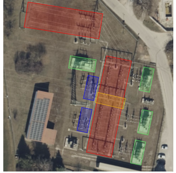
Figure 3: In the substation in Ettringen the busbar is split into multiple sections (redbox)
