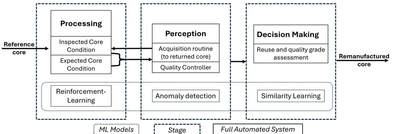
**Figure 10.** A scheme of core condition assessment through image and point cloud analysis, detecting quality deviations like corrosion or missing parts, which are then compared to expected conditions to determine reusability and quality grade (recreated from [32]).
