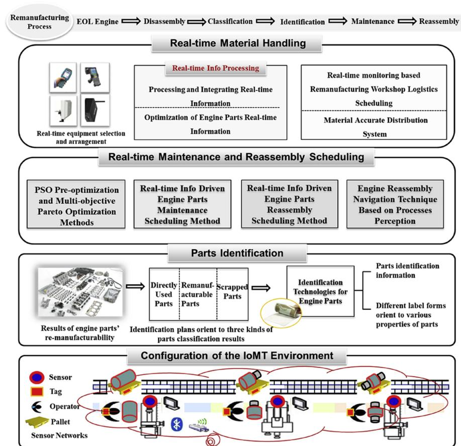
Figure 6. IIoT-integrated scheduling model for engine remanufacturing (adopted from [125]).
