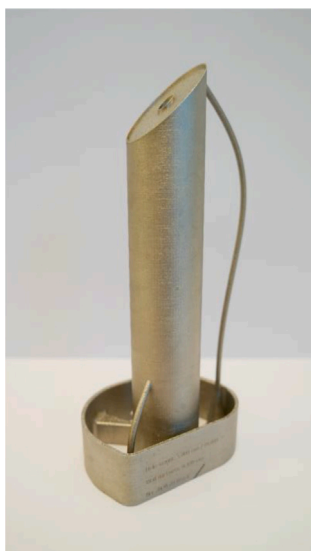
Fig. 3. Picture of a manufactured single version HeliDist unit with 10 turns and a channel height of 5 mm.
