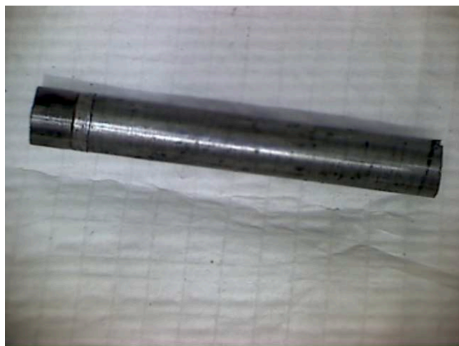
Fig. 5. Irradiated plenum section of fuel rod segment N0204.
