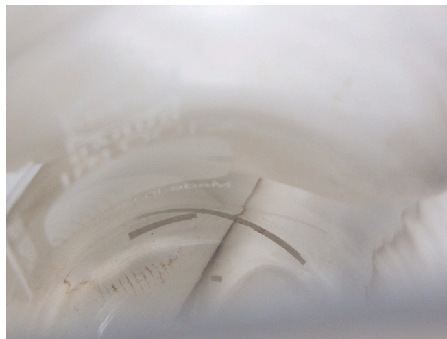
Fig. 6. Residual ZrO 2 layer after acidic digestion of the cladding specimen.
