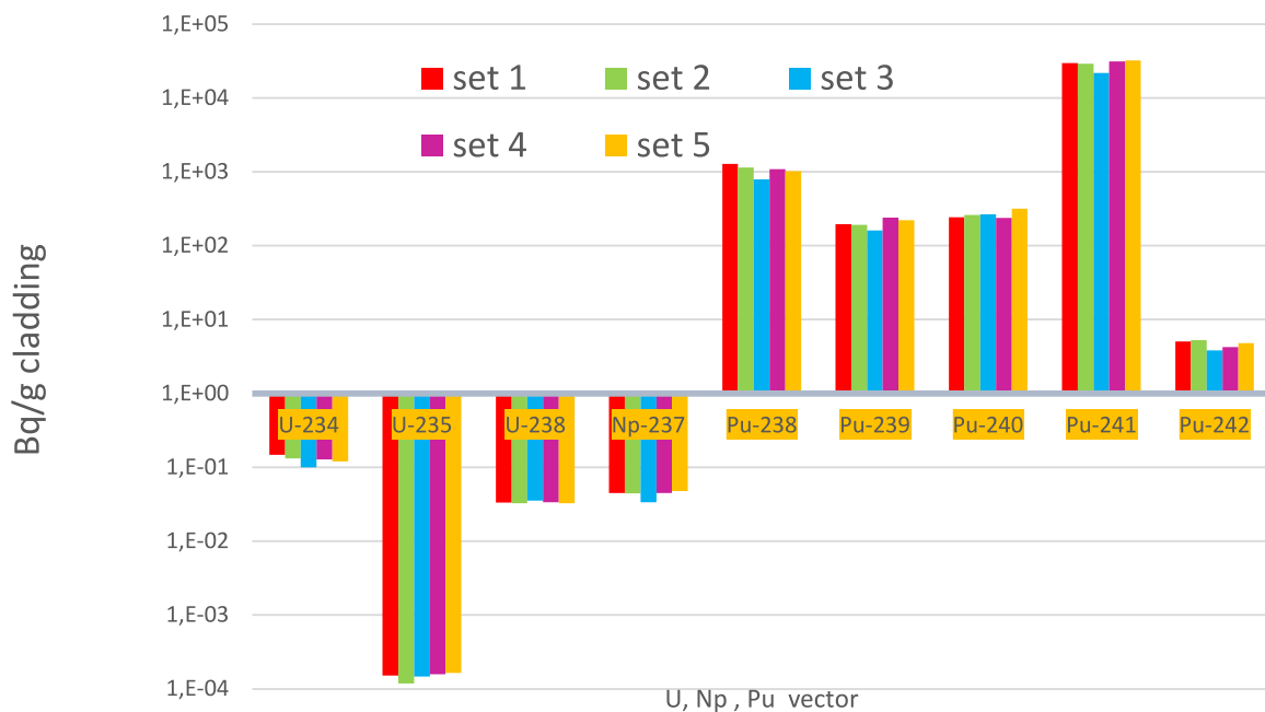
Fig. 3. Log-based simulation results for the uranium and plutonium vector of the benchmark.
