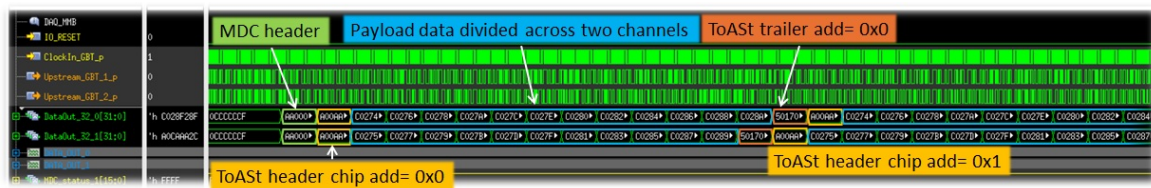
Figure 2. Data distribution across two upstream data links to optimize e-link bandwidth. The data format includes: an MDC header with event number details, a ToAST header identifying the ToAST under readout, the payload data packets, a ToAST trailer indicating the number of channels with events and a CRC (Cyclic Redundancy Check) for error detection, and an MDC trailer reporting the internal status of the MDC.
