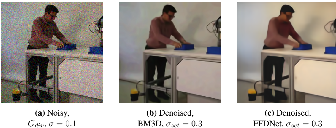
Figure 6.9: Visual comparison of the denoising results from BM3D and the custom-trained FFDNet with \sigma_{set} = 0.3 for an image corrupted with G_{div} of strength \sigma = 0.1 .
