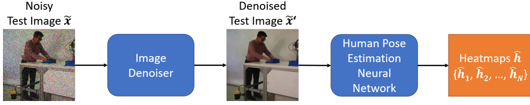
Figure 6.5: Depiction of the pipeline used after training when a dedicated image denoiser is employed. A (potentially) noisy test image is first denoised by the image denoiser. The resulting denoised image serves as input for the human pose estimation neural network.
