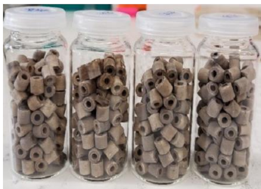
Figure 6: Photograph of four batches of synthesized Pt/Al 2 O 3 with optimized immobilization procedure of chemically reduced colloidal nanoparticles onto hollow cylinders. Synthesis conditions: Batch procedure, PVP:Pt ratio = 5 g PVP g Pt -1 and NaBH 4 :Pt ratio = 0.31 mol NaBH 4 mol Pt -1 .
