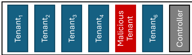
Figure 6.1: System model of a multi-tenant FPGA in a cloud environment. The FPGA is divided into a static partition responsible for management tasks and multiple tenant regions (PRRs), one of which is occupied by a malicious tenant attempting a power-hammering attack.
