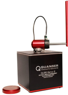
Figure 3.6: A Furuta pendulum as distributed by the Quanser company (QUBE™ Servo 2). Image source: https://www.quanser.com
