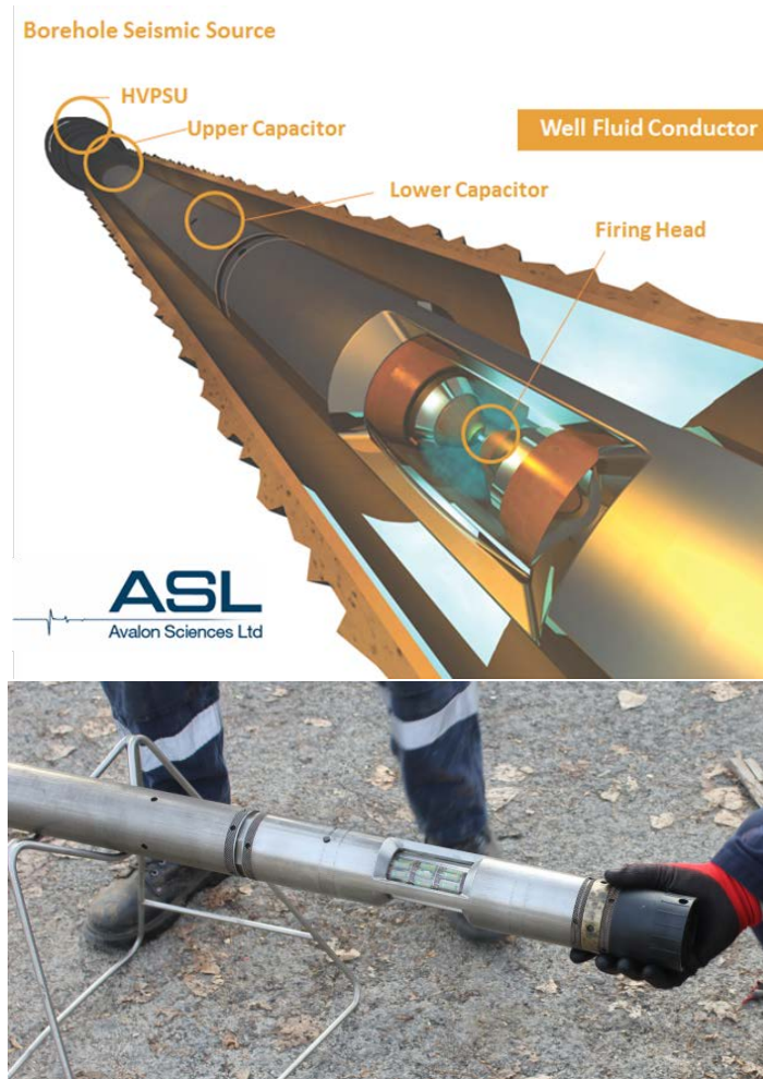
Figure 1-5: Advanced Sparker Tool (AST) of Avalon Sciences Ltd. Source: https://avalonsciences.com/
