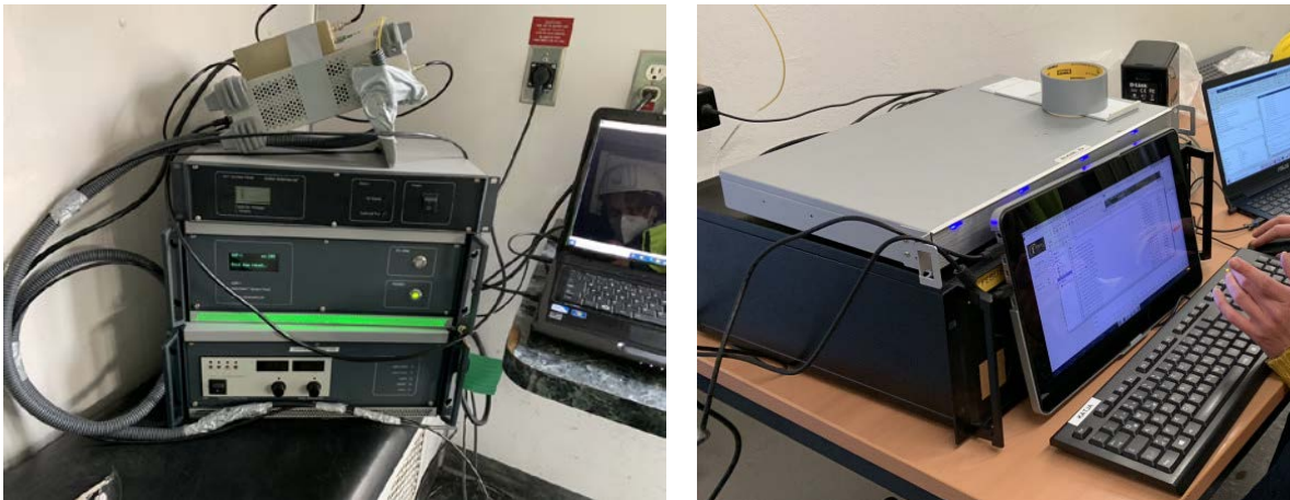
Figure 3-7: AST control panel in the wireline truck, with fibre stretcher used for the recording of time-break signals on the top (left). DAS-unit, data-storage device and Pc-Febus in the control room (right).
