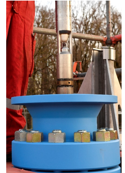
Sarker impulse probe from Avalon Sciences Ltd. (Photo: Marcus Schlaf)
