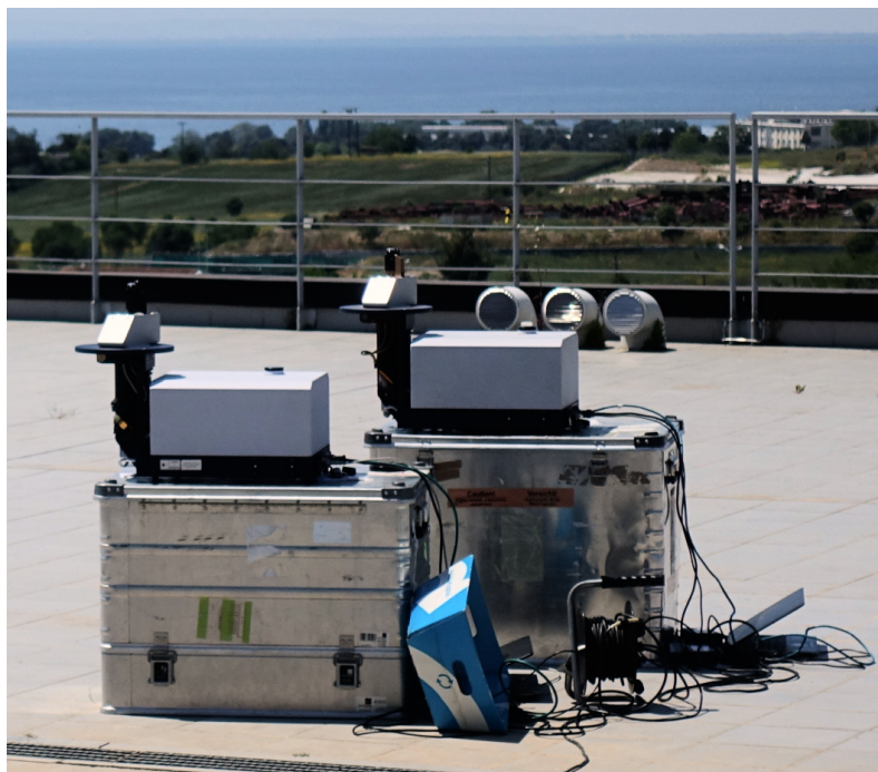
Figure 2.9.: Two EM27/SUN spectrometers operated side-by-side for calibration. The measurements were taken in Thessaloniki in 2022 for calibration. The spectrometers can be carried by two persons. Photographed by Lena Feld.
