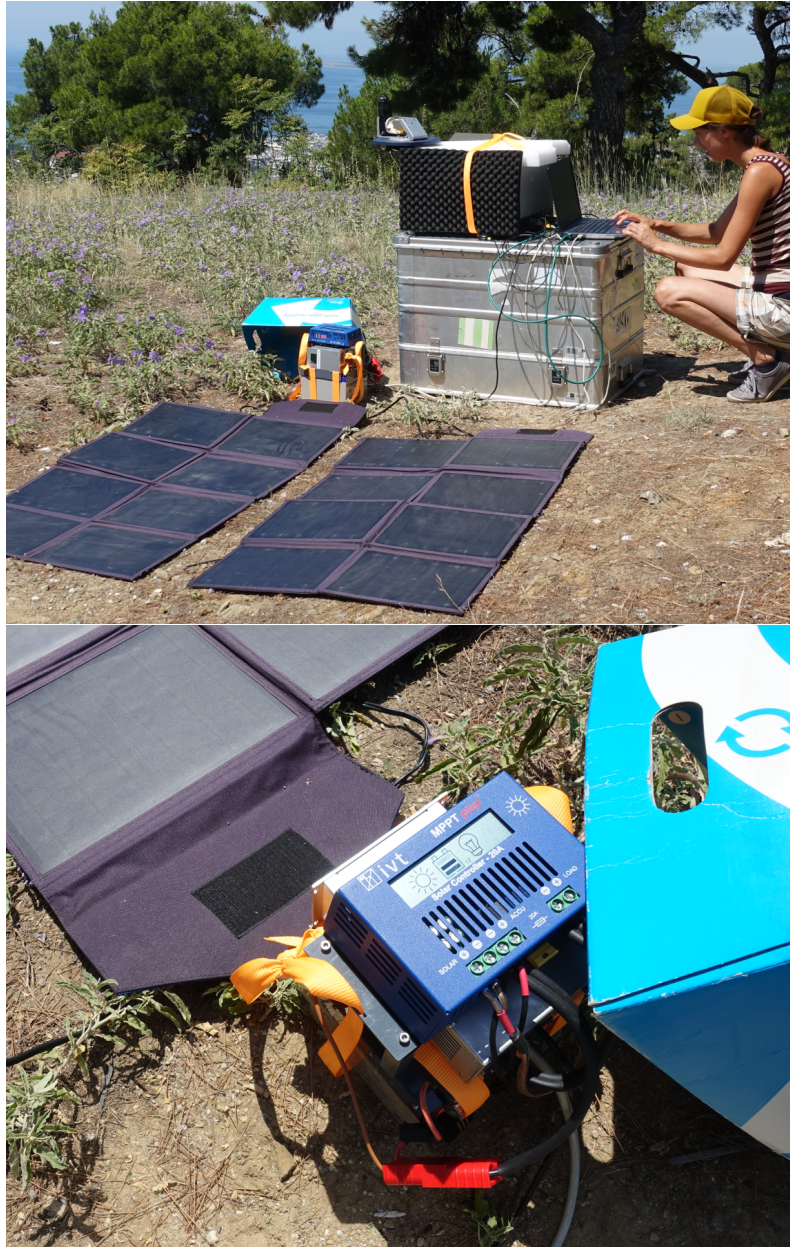
Figure 3.2.: Portable setup of SN96. The pictures show the setup that allowed mobile deployment of SN96 on a daily basis. The first image shows the whole setup, with the solar panels in the front, and the spectrometer in operation in the back. The spectrometer is shielded from sunlight with foam. The small box next to the spectrometer is shown in more detail in the second image. It contains the electronic control of the power supply and the buffer battery. Photography by Pablo Schmid and Lena Feld.
