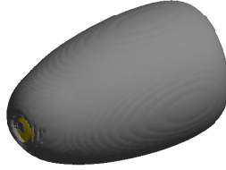
Figure 5.52: Instantaneous wake structure for flow around a fixed isolated sphere at Re = 300 , Ma = 0.8 , TR = 2 given by the isosurface of the second invariant of the velocity gradient tensor given by QD_p^2/u_\infty^2 = 1 \times 10^{-4} .
