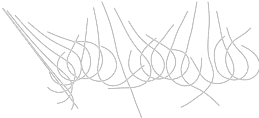
Figure 5.9.: Snapshots of the flight motion of the flying spaghetti (10 LCS3 elements) in increments of \Delta t = 0.5 from t = 0 to t = 10 .
