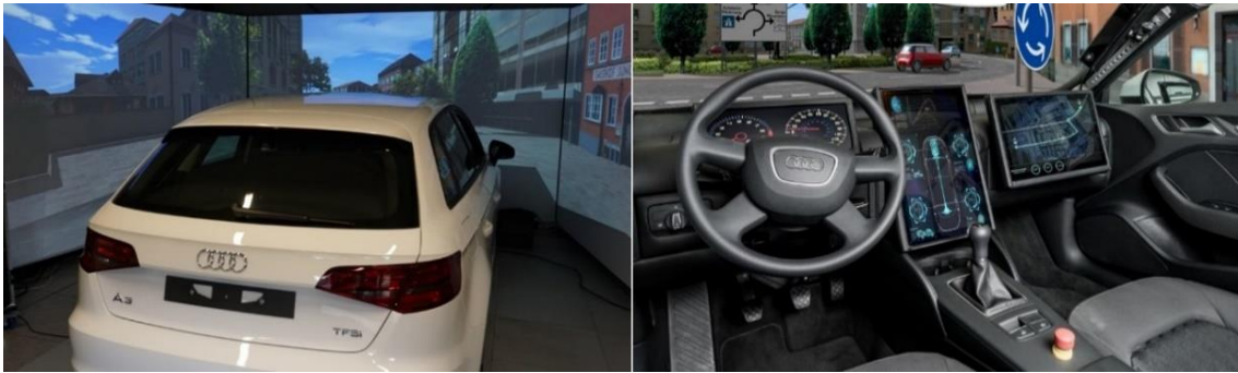
Figure 28. Driving Simulator frontal projection screens (left) and interior of the simulator vehicle (right) (Ehrhardt, Martin, et al., 2024)
