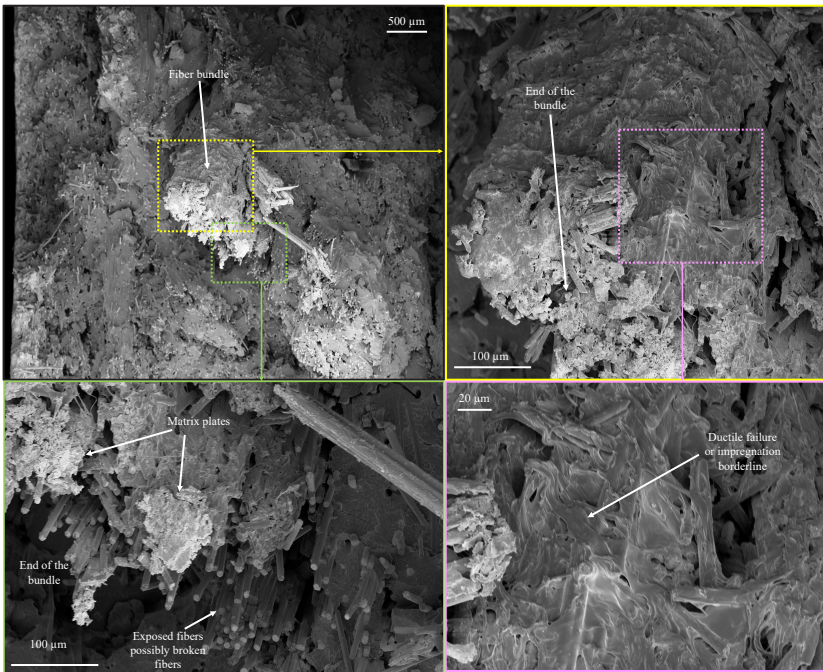
Figure 5.23: SEM pictures of the fracture surface of the 0° CF LFT flow specimen from Figure 5.21 at the point of local strain increase marked in Figure 5.21 in different magnifications.
